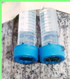
Fig. 2. Sugar water monitors consists of 50 ml centrifuge tubes (15 ml tubes shown in photo) filled with 25% sugar water. The cap has a hole drilled in its center and is screwed down over a piece of Weedblock. This material has many tiny holes through which the ants can drink.
