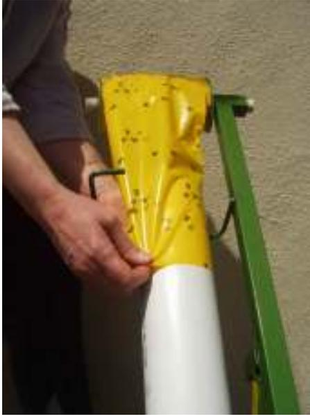
The Magnum Insect-A-Peel Assembly holds a reel with a 50 foot long tube of yellow sticky plastic. Two brackets hold a 29 inch long by 3 inch diameter PVC pipe. The plastic tube slides easily over the tube and fastens to a take-up reel at the bottom of the unit. A heavy-duty socket holds the unit horizontal or at a 45° angle on a 30 inch post.
